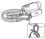
Pass the ends of the shoulder strap through the strap mount on the grip belt and adjust the length of the strap.
